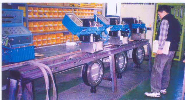
Teflon coated body with titanium disc
